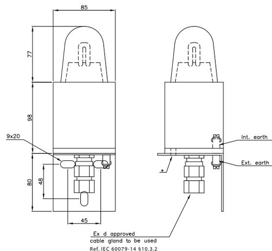
\* For disassembling the top section (tube and dome) the locking screw must be screwed at least 2 turns counter clockwise. Use a 4mm hex Allen key for TNFCD, 3mm for TNFCDM
